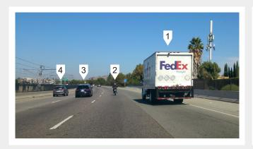
Multiple targets acquired in a 120° field of view. Multiple arrays can be assembled to yield 360° scanning and tracking.
